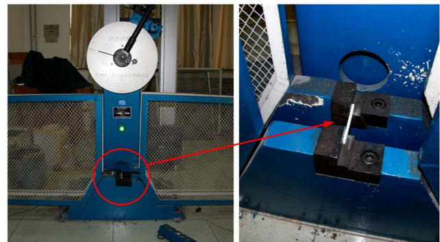
Fig. 7 Charpy pendulum impact resistance test
